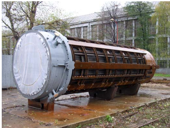
Fig. 10 Tube Bundle of Vertical Steam Cooler with Floating
