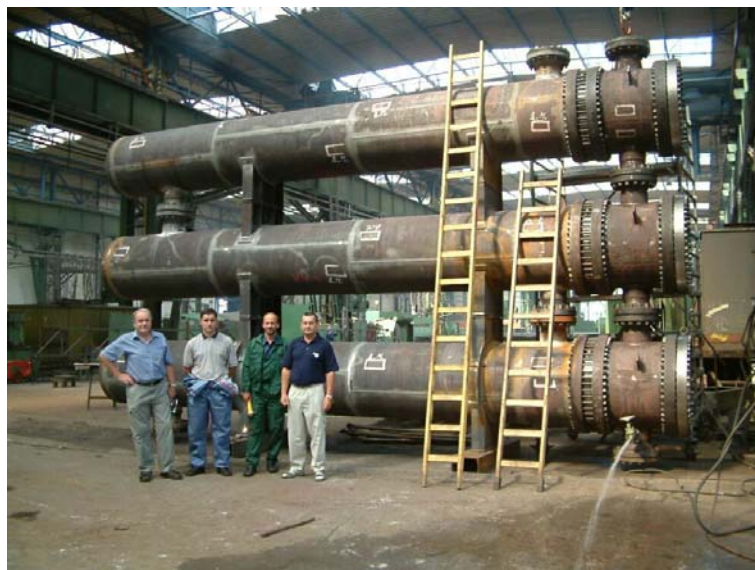
Fig. 1 Heat Exchangers for Petrochemical Unit
