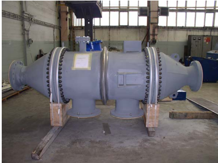
Fig. 7 Heat Exchanger with Fixed Tubesheets and Shell Expansion Joint Resp.
