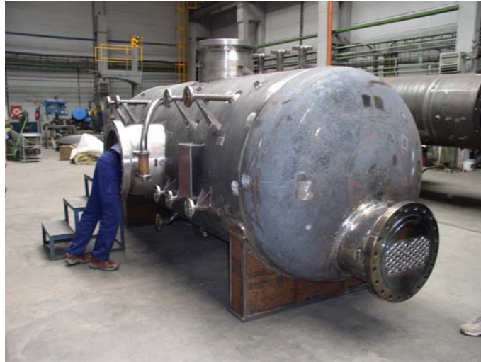
Fig.4 Heat Exchanger / Boiler with Steam Generation
