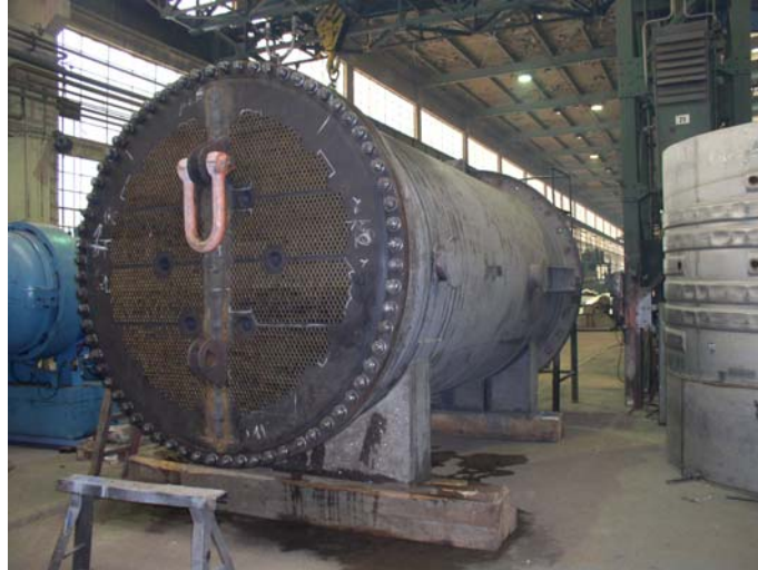
Fig.5 Bundle of Heat Exchanger with Condensation
